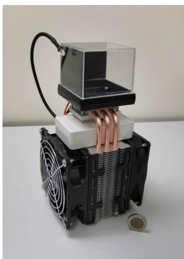
Fig. 1 Cloud chamber using Peltier coolers.
