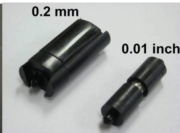
The larger and smaller weight is for measurement in 0.2 mm and 0.01 inch for each flip of the tipping buckets. Settings in WeatherLink and console mismatch with the actual installed mass would give underestimated/overestimated amount of precipitation.
