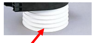
Radiation shield with temperature and humidity sensor inside
