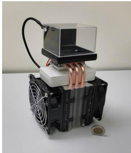
Fig. 1 Cloud chamber using Peltier coolers.
